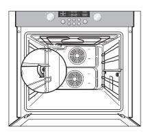
2. Remove the screw at the front by turning it anti-clockwise after latching the side runner.
